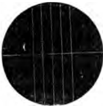
ARRANGEMENT OF WIRES IN A TRANSIT INSTRUMENT.
